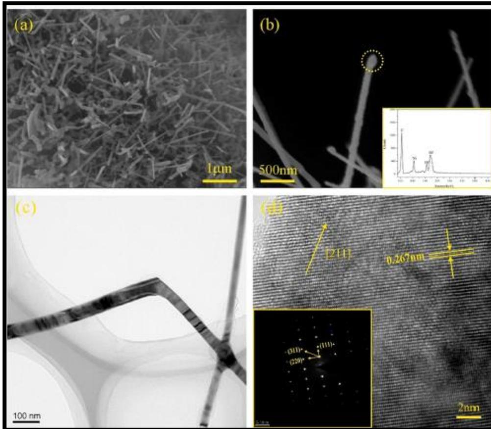
**Figure 4.5: HfC nanowires synthesis**
