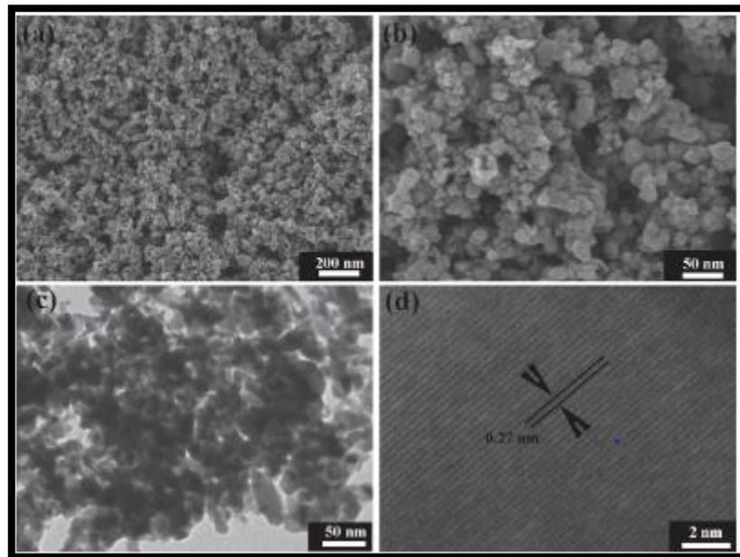
**Figure 4.3: SEM Image of HfC after Solid-state-Reaction**
