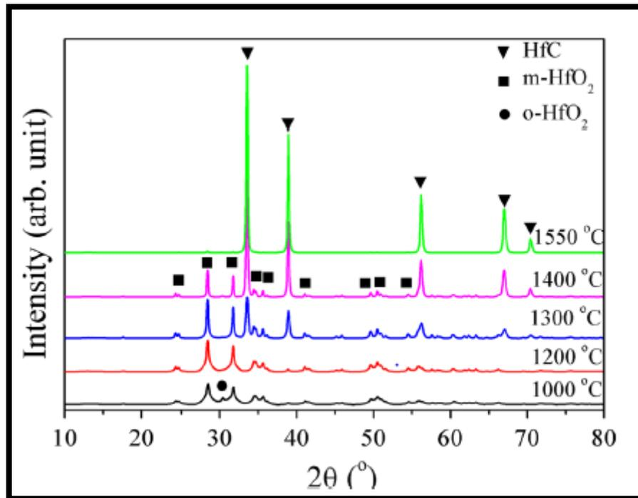
**Figure 4.4: Intensity of HfC at different temperature**
