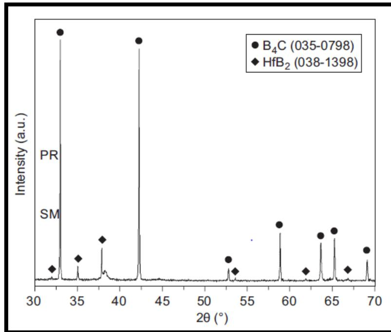
**Figure 2.2: X-ray Diffraction of Hafnium compound**
