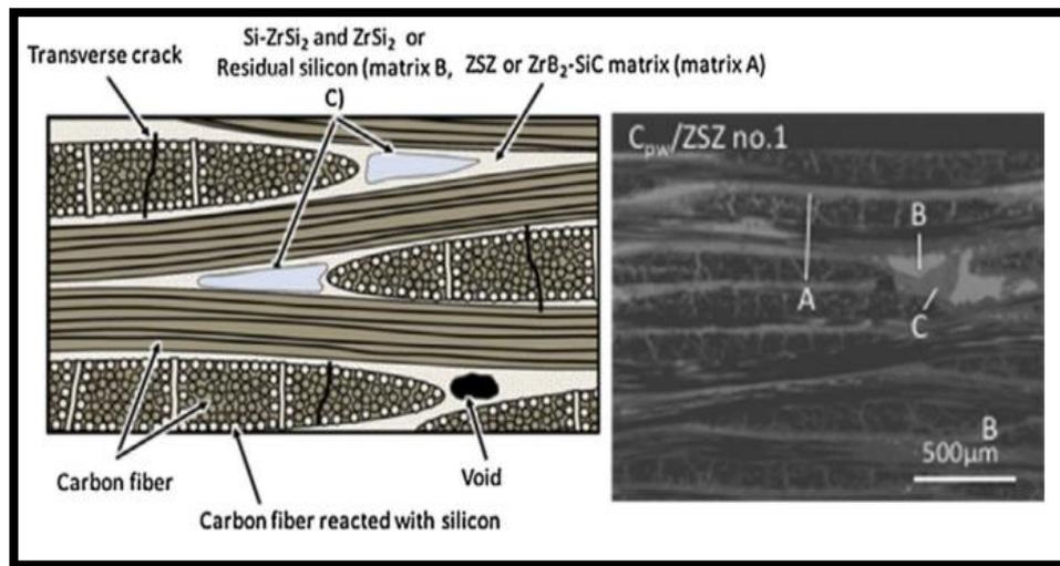
**Figure 1.2: Microstructure of ceramic composites**
