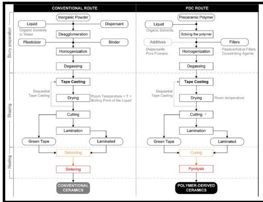
**Figure 2.6: Conventional and PDC Methods**
