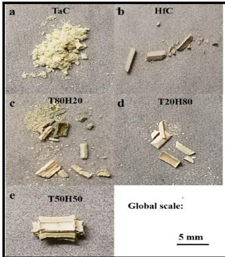
**Figure 4.2: Post-oxidation samples of different combination**
