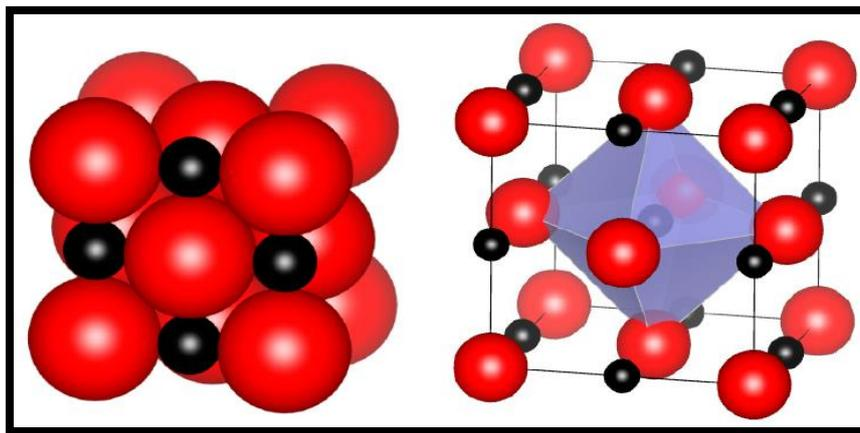
**Figure 1.1: Structure of rock salt**
