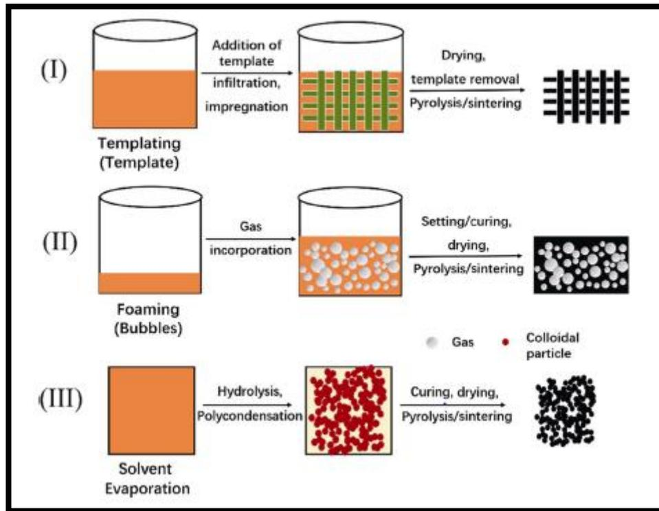
**Figure 1.3: Sol-gel; Method of HfC manufacturing**
