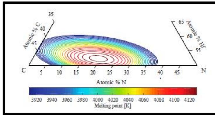
**Figure 2.3: Melting Point of atomic C and Hf**
