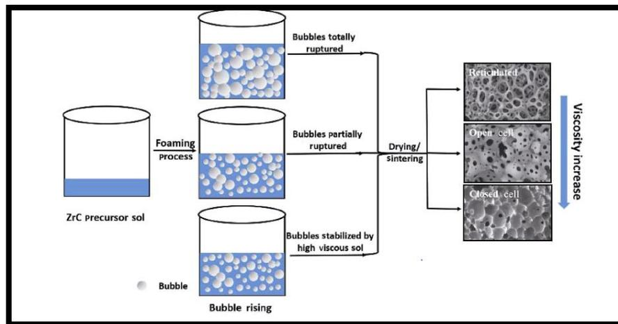
**Figure 2.4: Bubble Growth and Stabilisation Process**
